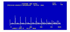
Autocorrelation MOD of unknown signal after FFT shows it to be a 50 Baud signal
