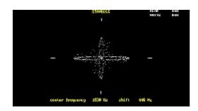
Straddle showing a tuned RTTY signal
