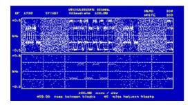
Oscilloscope showing four frequency Twinplex signal
