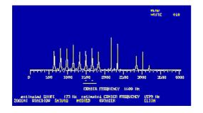
0 - 3800 Hz Audio Spectrum Analyzer showing VFT signal (J7B)
