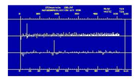
AutoCorrelation Bit module showing 100 Baud Sitor B with 35 element repetition. Top screen half shows bits from 0 to 512, Bottom half is the frist 100 bits 'zoomed' in.
