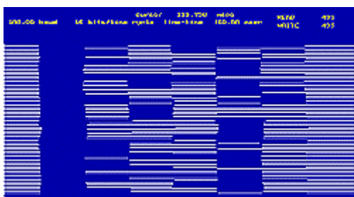
Speed Bit module showing Asynch. 7 1/2 element of 50 Baud Baudot signal
