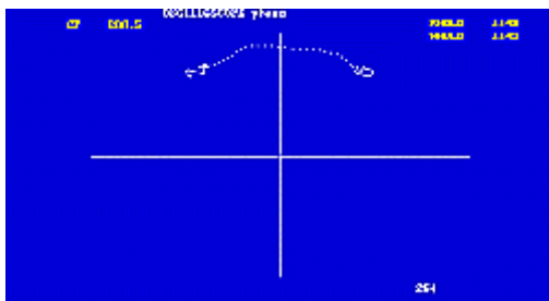
Phase display module showing PSK on 198 kHz Radio 4
